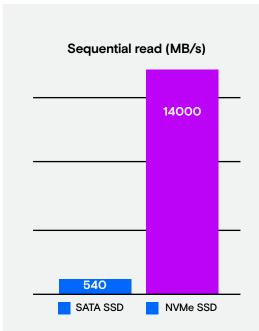
Figure 1: Sequential reads Micron 9550 NVMe SSD vs. Micron 5300 SATA SSD<sup>2</sup>.
